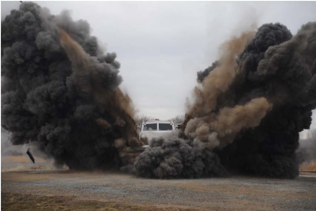
Protector 2 in 15 lb TNT Blast 28 January 2010
