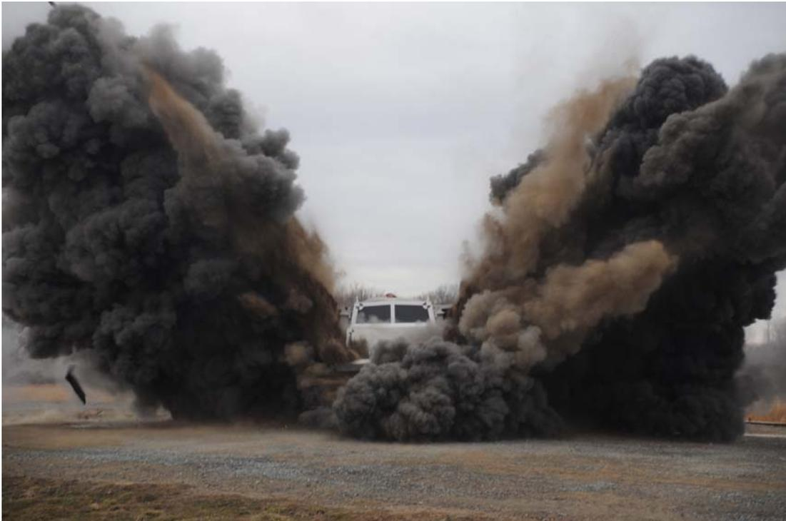
An internal overpressure of only 2.3 psi was recorded during the blast and the front of the vehicle lifted only 2 ft vertically during the blast. Hull deformation was minimal and there were no hull or transfer case cover breaches nor did any shrapnel enter the crew compartment.
